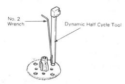
To make the above adjustments, use the 3/16" socket end of the dynamic half cycle tool to loosen the locking nut, then insert the end of the No. 2 splined wrench, (T11-21) through the slot on the side of the tool to turn the ribbon lift height adjusting screw.
